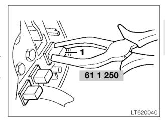
• Grip indicator lamp (1) diagonally with relay pliers, BMW No. 61 1 250, and pull out or press in.
