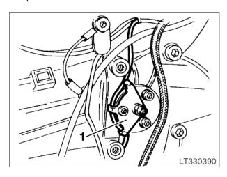
• Install bracket (1) for line of electric side stand switch.
