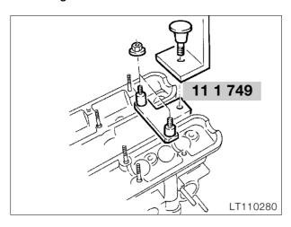
Screw support plate, BMW No. 11 1 749, for the valve spring clamping tool on to the rear of the cylinder head.
