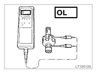
Measure resistance between slip rings and armature.
