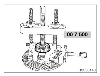
Remove taper roller bearing from ring gear with puller, BMW No. 00 7 500.
