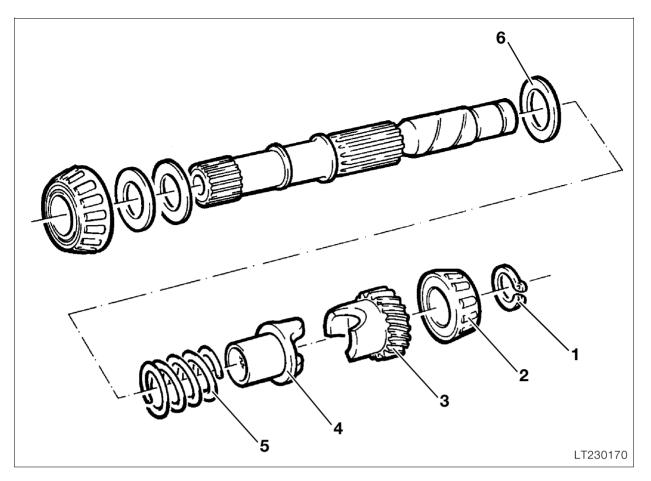
Disassembling and assembling input shaft
