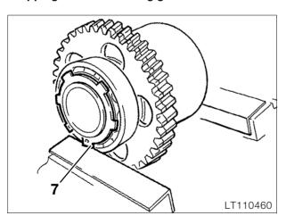
Clamp the damper housing into a vise with soft jaws, to take the load off circlip (7).
