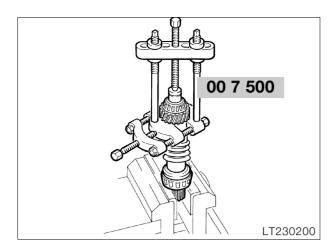
• Fit universal puller under the spur gear and pull down taper roller bearing as far as it will go on the retaining ring.
