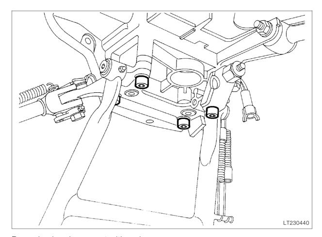
Removing bearing mount with main stand
