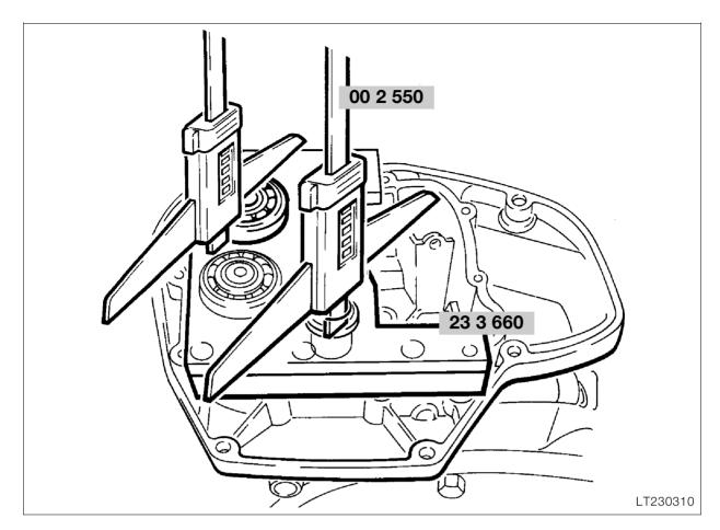
Measuring distances between transmission shafts
