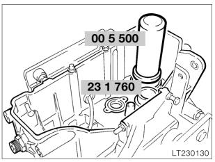
Fit shaft sealing ring using drift,
