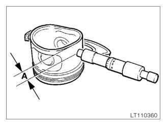
Measure piston diameter with a micrometer at distance "A".
