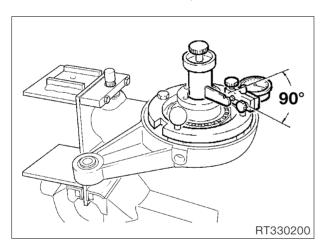
With the palm of the hand, press crown wheel into housing and check gear backlash by turning backward and forward.
