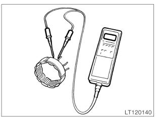
Check winding outputs individually with respect to earth.
