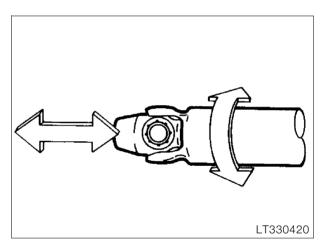
Determine axial and radial play by shifting axially and turning radially.
