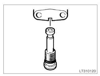
Release bottom screw fitting and pull out fixed tube.
