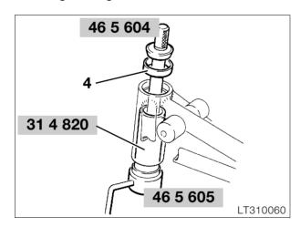
• With the aid of the spindle of the frame test gauge, BMW No. 46 5 604/605, in conjunction with the thrust piece, **BMW No. 31 4 820**, install bearing outer race (4) together with hexagon nut and washer to the limit stop.
