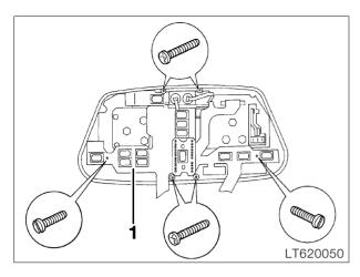
• Release securing screws and carefully lift out p.c. board (1).
