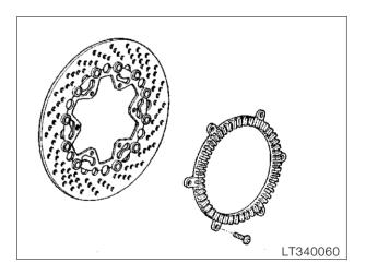
• Release pulse wheel on brake disc carrier.
