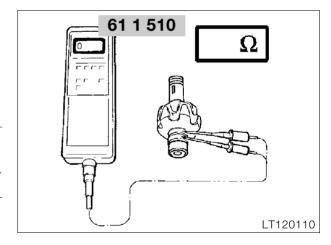
Using the test probes of the BMW diagnosis tester, BMW No. 61 1 510, measure the resistance across the slip rings.
