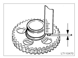
Measure distance "a" from ball bearing seat to tensioning gear.
