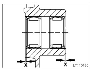
Press the needle roller bearing into the freewheel gear so that distance (x) is the same at both
