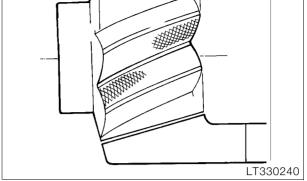
If this contact pattern is obtained, a thinner spacer ring must be installed.
