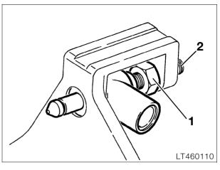
• Loosen locknut (1), unscrew pressure screw (2).
