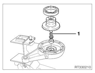
Take up excessively large gear backlash by fitting a thin spacer and too little gear backlash by fitting a thick spacer (1).
