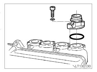
Tightening torque: Intake stub pipe ...... 9 Nm
