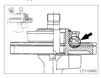
Place a suitable spacing washer (arrow) on the tensioning gear.
