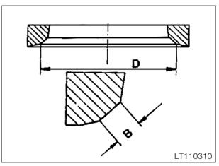
D = valve diameter B = valve seat width
