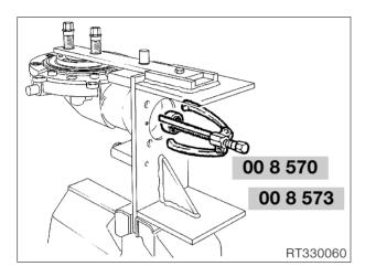
Remove outer race of needle bearing with the aid of inner extractor, BMW No. 00 8 573, and support, BMW No. 00 8 570.
