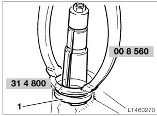
Remove outer bearing race (1) at top and bottom with inner extractor, BMW No. 00 5 560 in conjunction with support ring, BMW No. 31 4 800.
