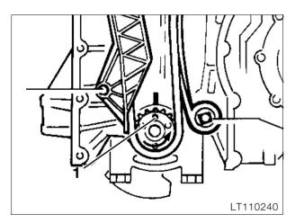
Set cylinder 1 (timing end) to TDC, noting direction of rotation (arrow). Pin (1) on the crankshaft must be aligned with the marking on the housing.
