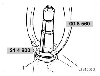
• Remove bearing outer race (1) using extractor BMW No. 00 5 560 (2), and support ring BMW No. 31 4 800 (3).
