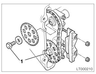
Release retaining bolts of sprockets and remove sprockets.
