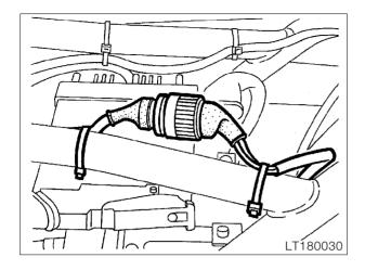
Separate plug connection for oxygen sensor.
