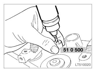
• Fit drilling bushing (1), **BMW No. 51 0 500**, in hole.
