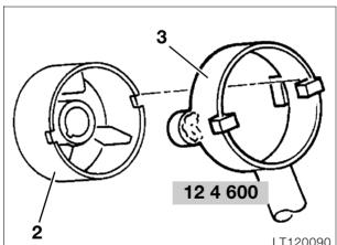
Tightening torque: Coupling housing......50 Nm
