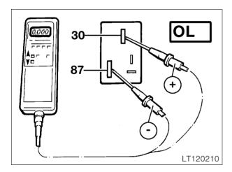
Connect positive lead from measuring instrument to terminal 30, negative lead to terminal 87.
