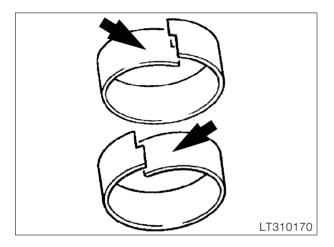
• Slightly preform new plain bush in order to achieve an optimum fit on the fixed tube.
