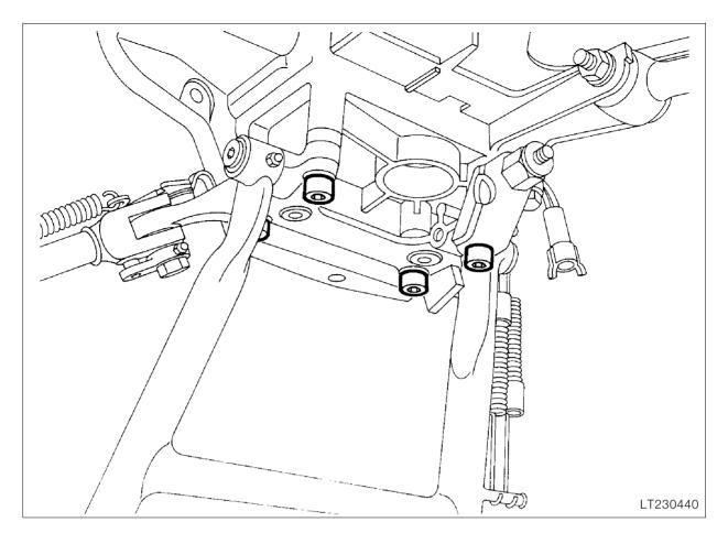
Installing bearing mount with main stand
