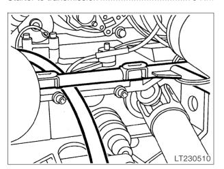
• [ABS I] Install support bracket for pressure modulators.
