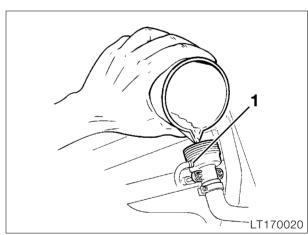
• Fill with coolant up to lower edge of filler neck (1).
