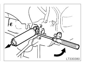
• Press off drive shaft with screwdriver.
