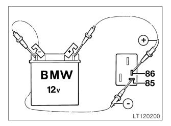
• Connect terminal 86 to positive battery terminal, terminal 85 to earth (ground).
