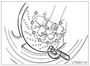
Measure thickness of brake disc with a micrometer.
