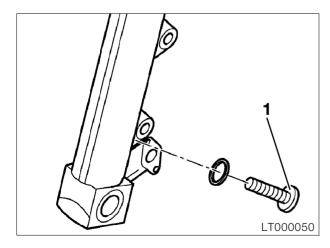
Release left and right oil drain plug (1).
