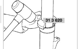
• Fit drift, **BMW No. 31 3 620**, on to fixed tube and release.
