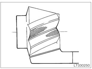
If this contact pattern is obtained, a thicker spacer ring must be installed.
