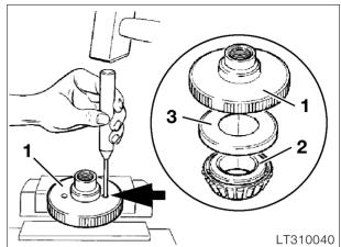
Using a drift, knock out taper roller bearing together with dust ring (2,3) out of setting ring (1).
