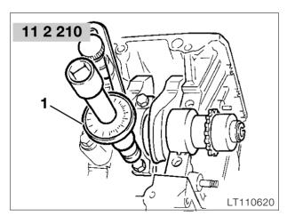
Tighten the big end bearings with wrench angle indicator (1), BMW No. 11 2 210.
