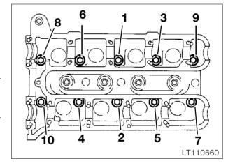
Tighten the cylinder head bolts in the order shown.
