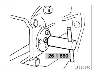
Coat bearing pin of fixed bearing with Optimoly TA and install and firmly tighten with special tool BMW No. 26 1 660.
