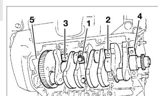
Tighten the bearings in the order shown, starting from the centre and working outwards.
