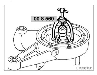
Remove outer bearing race with internal extractor, BMW No. 00 8 560.
