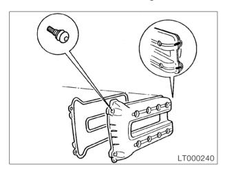
• Insert gasket into cylinder head cover.
