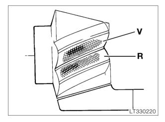
If the correct spacer ring is installed, the no-load contact pattern as shown above should be obtained.
