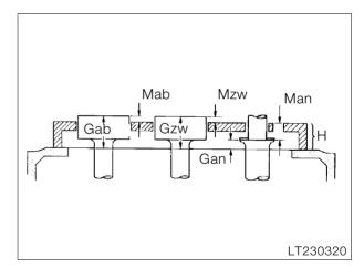
Mab = Dimension output shaft to measuring plate
