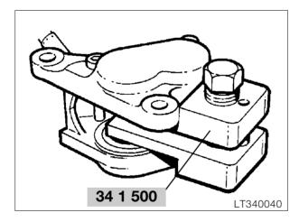
Use piston resetting tool, BMW No. 34 1 500, to press the brake piston fully back.
