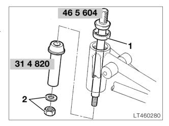
Fit outer bearing race (1) top/bottom with spindle, BMW No. 46 5 604, from frame test gauge, BMW No. 46 5 600, and spacer,
