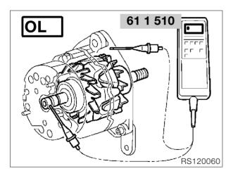
Measure resistance between sliprings and armature.
