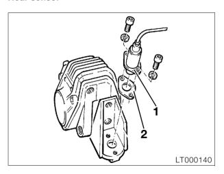
Check sensor spacing with feeler gauge.
