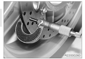
Measure the thickness of the brake discs at several points with a caliper gauge.
