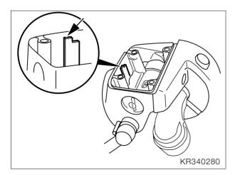
Top up the brake fluid level to the "MAX" mark (arrow).
