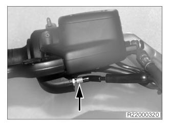
Use the adjusting screws (arrow) to adjust play of the throttle cables.
