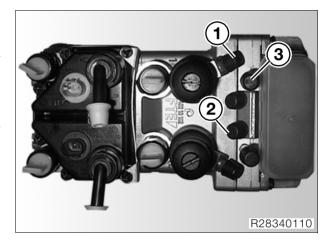
Connect the brake bleeding device to bleed screw (1) of the front metering cylinder, but do not switch on.
