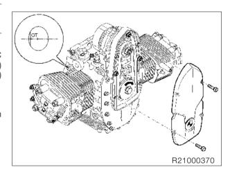
Select a gear and turn the rear wheel, or set the piston to TDC on the ignition stroke by turning the belt pulley.
