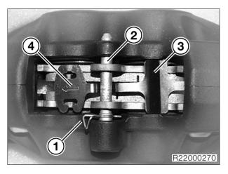
Remove the split-pin keeper (1) from grub screw (2). • Remove grub screw (2) and spring (3).
