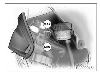
• Top up the brake fluid level to the "MAX" mark.
