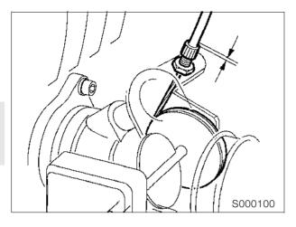
Turn the adjusting screws to adjust the play of the cables for the left and right throttle valves.
