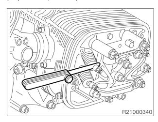
Check valve clearance with feeler gauge and, if necessary, correct with adjusting screw.
