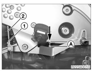
Set the adjusting screw of the footbrake lever to distance A.
