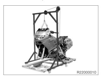
Using the straps, secure the front of the motorcycle to the assembly crane, BMW No. 46 5 640.
